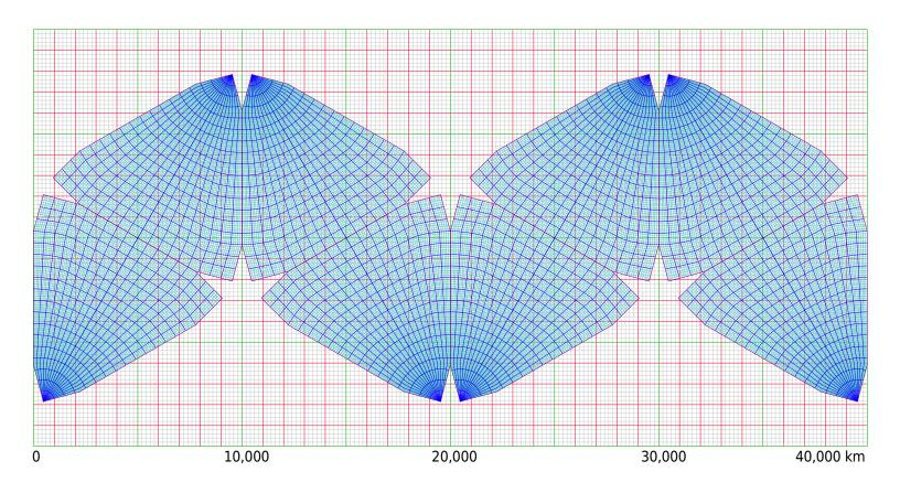
Cahill-Keyes Octant Graticule with one-degree geocells Scale 1 1/200,000,000 2010-08-17 printed from OOo Draw 2.0
